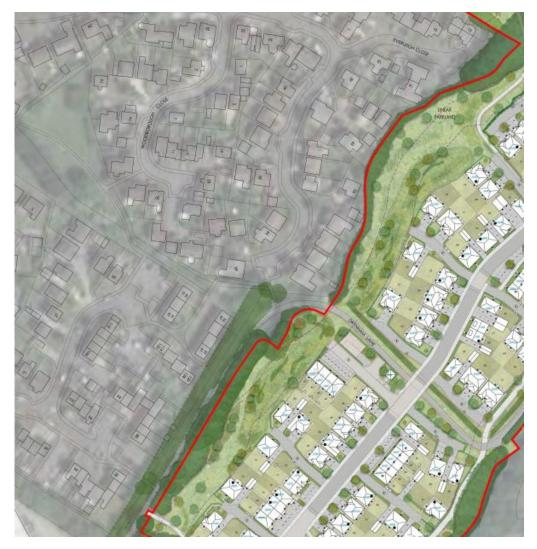
A previously proposed footpath has been removed behind the properties of Lydiard Way at the request of the neighbours and the unitary ward Councillor. A request to move the attenuation ponds further away from these properties was not however possible due to the location of the existing sewer pipes.
